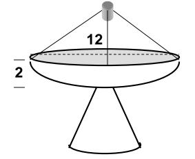
A satellite dish is in the shape of a parabolic surface. The dish is 12 ft in diameter and 2 ft deep. How far from the base should the receiver be placed?
