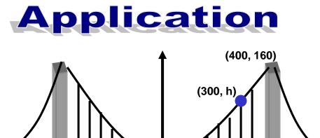
The towers of a suspension bridge are 800 ft apart and rise 160 ft above the road. The cable between them has the shape of a parabola, and the cable just touches the road midway between the towers.
